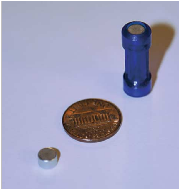
Figure 1. Magnets embedded in a plastic piece (right) from a toy set can easily detach and are small enough to be swallowed by a child.
