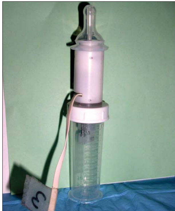
Figure. Sucking device. The block with the built-in transducer is inserted between the bottle and the nipple. The cable connects to the digitalizer.
